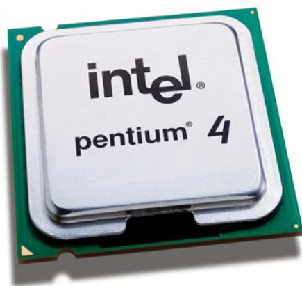
Figure 6-8. Intel Pentium 4 32-bit microprocessor.
