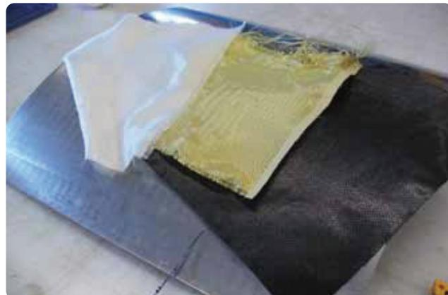
Figure 3-8. Fiberglass (left), Kevlar® (middle), and carbon fiber material (right).
