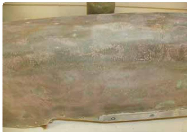
Figure 3-9. Copper mesh lightning protection material.
