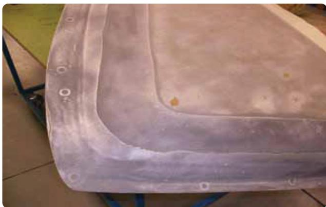
Figure 3-10. Aluminum mesh lightning protection material.
