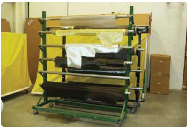
Figure 3-11. Dry fabric materials (top to bottom: aluminum lightning protection mess, Kevlar®, fiberglass and carbon fiber).
