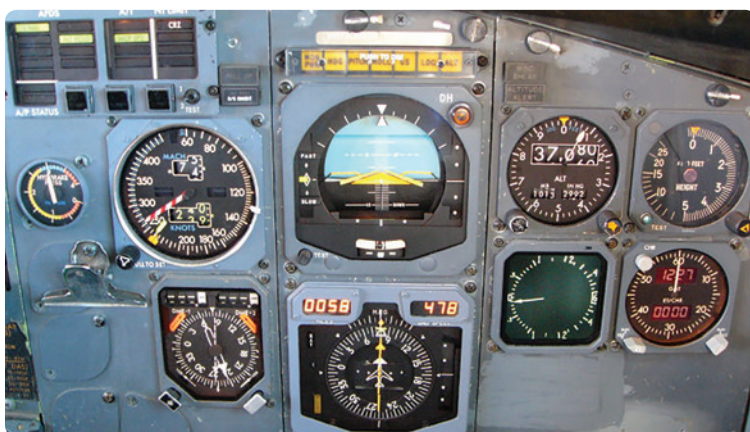
Figure 1-3. Equivalent Electromechanical Flight and Navigation Instruments on the left.
