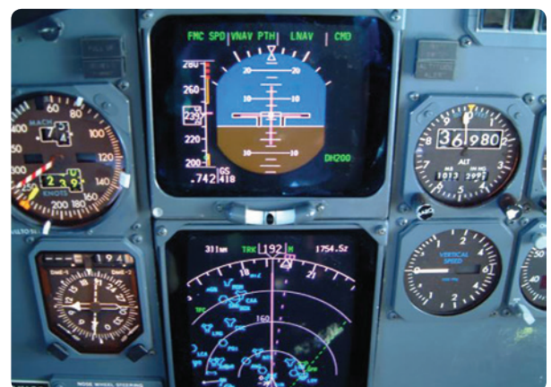
Figure 1-3. Equivalent Electromechanical Flight and Navigation Instruments on the left.
