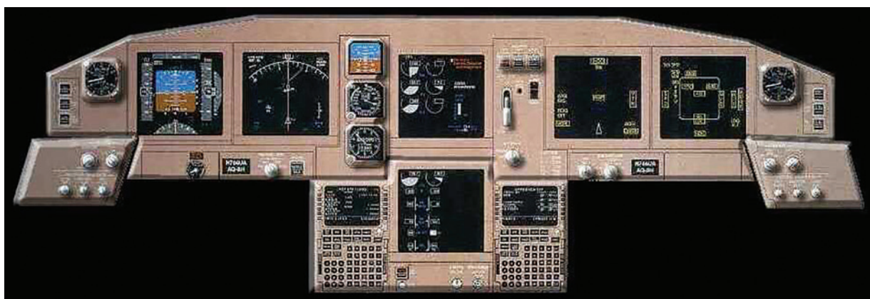
Figure 1-5. Electronic Displays are driven by Symbol Generators.
