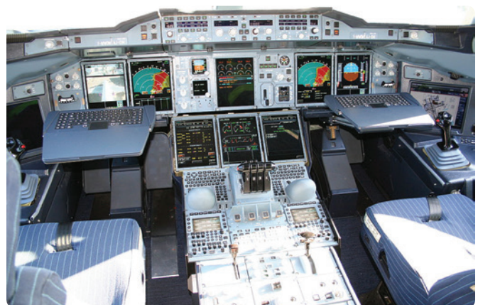
Figure 1-2. Airbus A380 EIS with 8 Large LCD Displays.
