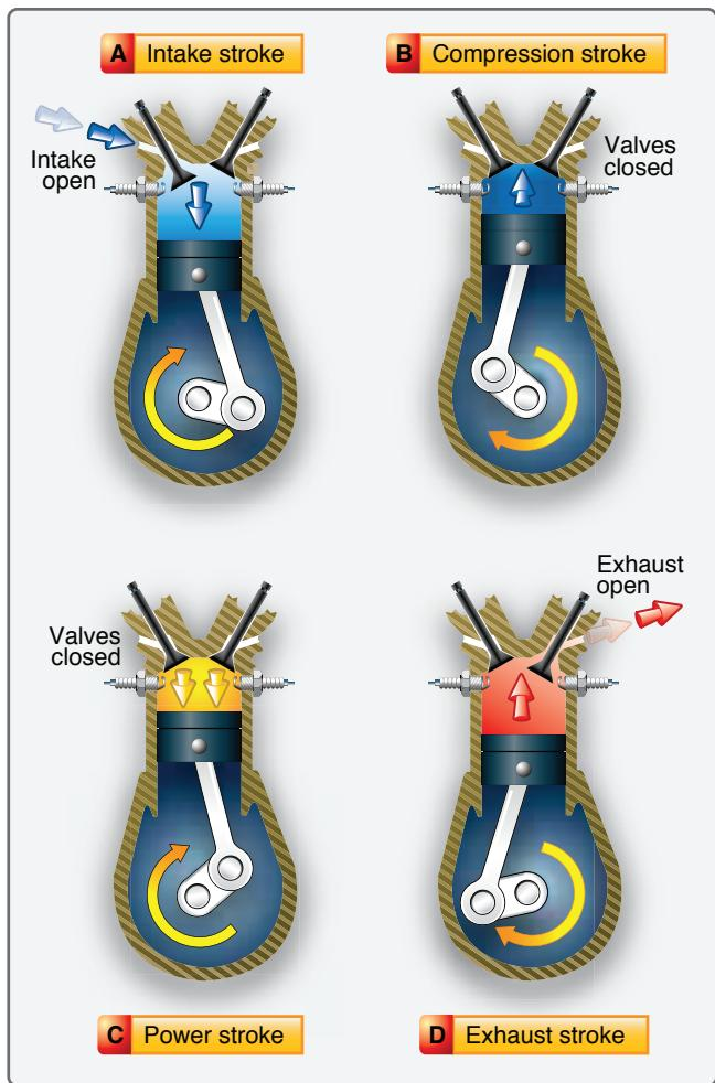
Figure 1-2. Four-stroke cycle.
