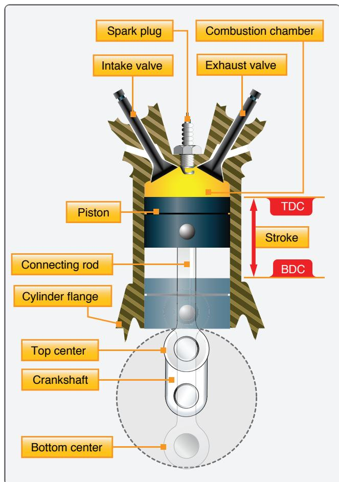
Figure 1-1. Piston engine design and components.
