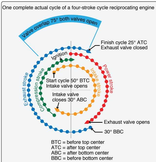
Figure 1-3. Four-stroke valve timing.
