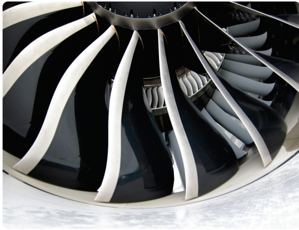
Figure 3-3. Inlet fan blades and guide vanes (inner circle) on a GENx engine.
