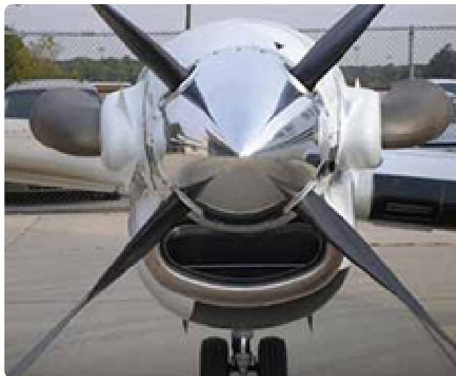
Figure 3-7. An example of a ducted arrangement on a Turboprop engine.
