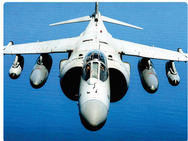
Figure 3-4. An example of a divided entrance duct.
