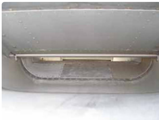
Figure 3-8. Deflector doors used to deflect ice or dirt away from the intake.
