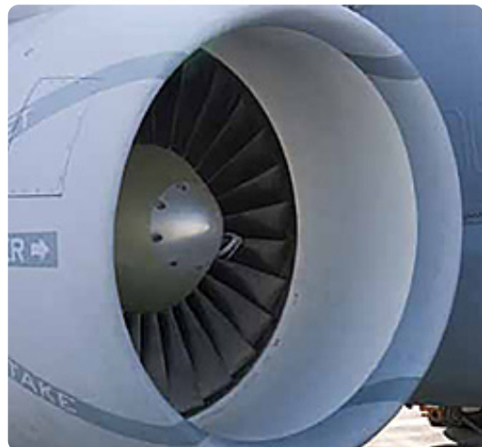
Figure 3-2. Typical turbofan inlet.
