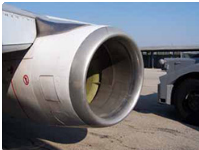
Figure 3-9. A typical turbofan intake section.
