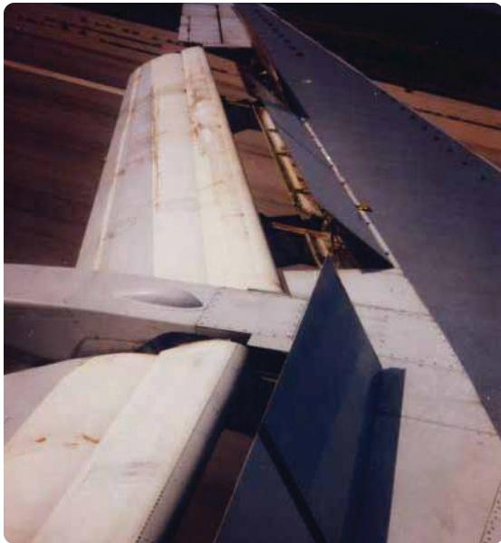
Figure 1-8. Spoilers deployed upon landing a transport category aircraft.
