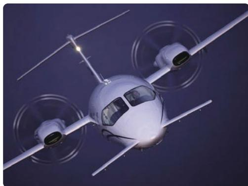
Figure 1-11. The Piaggio P180 includes a variable-sweep canard design, which provides longitudinal stability about the lateral axis.
