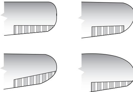
Figure 1-2. Aileron location on various wings.
