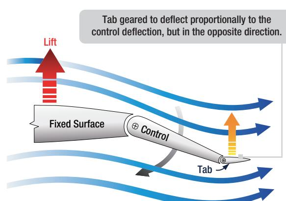
Figure 1-11. Balance tabs assist with forces needed to position control surfaces.
