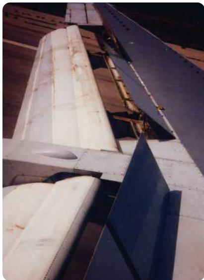
Figure 1-5. Spoilers deployed upon landing a transport category aircraft.
