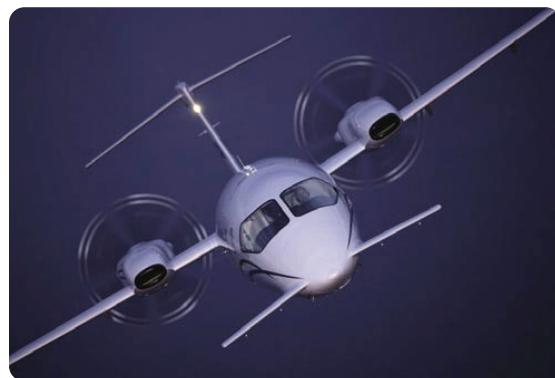
Figure 1-8. The Piaggio P180 includes a variable-sweep canard design, which provides longitudinal stability about the lateral axis.
