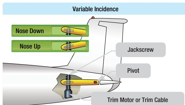
Figure 1-7. Some airplanes, including most jet transports, use an variable stabilizer to provide the required pitch trim forces.
