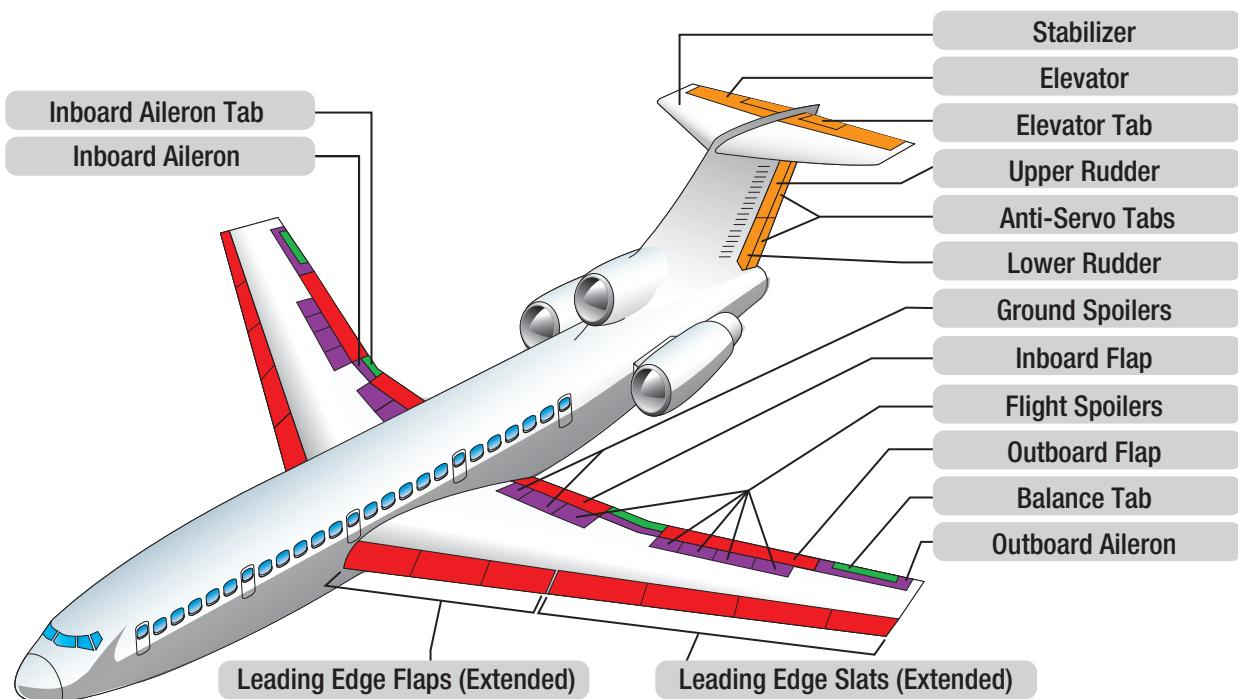
Figure 1-4. Typical flight control surfaces on a transport category aircraft.
