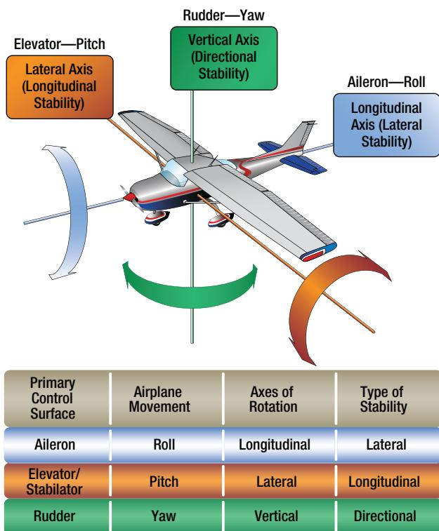
Figure 1-1. Flight control surfaces move the aircraft around the three axes of flight.
