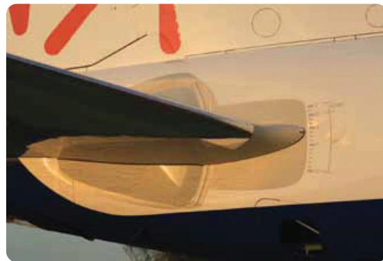
Figure 1-6. A stabilizer and index marks on a transport category aircraft.
