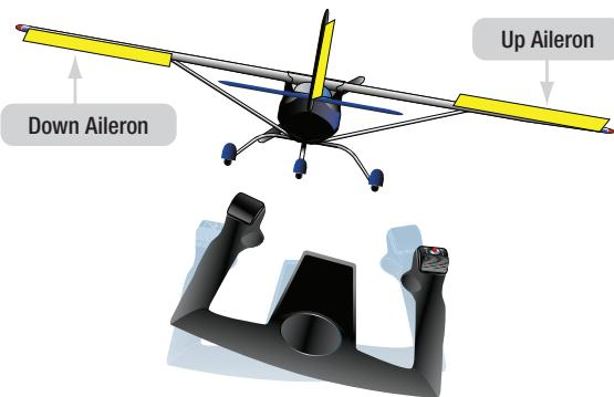
Figure 1-3. Differential aileron control movement. When one aileron is moved down, the aileron on the opposite wing is deflected upward.
